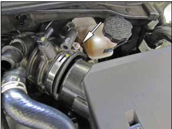
4. Loosen the hose clamp that secures the factory intake tube to the air filter housing.
