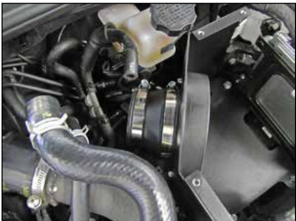
12. Install the step coupler onto the filter adapter and secure with the provided hose clamp.
