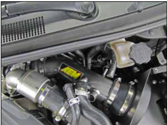
14. Install the intake tube into the couplers, align for best fit and then secure with the provided hose clamps.
