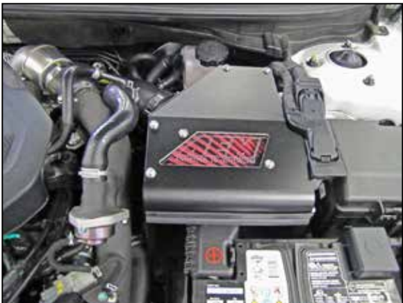
19. Install the heat shield lid onto the heat shield and secure with the provided hardware.
