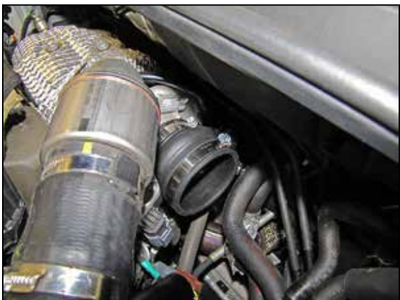
13. Install the hump coupler onto the turbo inlet and secure with the provided hose clamp.
