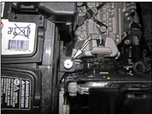
8. Install the rubber mounted stud onto the battery tray as shown.
