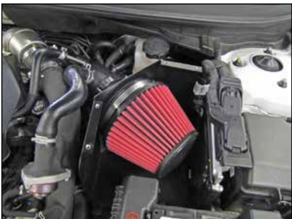
16. Install the AEM® air filter onto the filter adapter and secure with the provided hose clamp.
