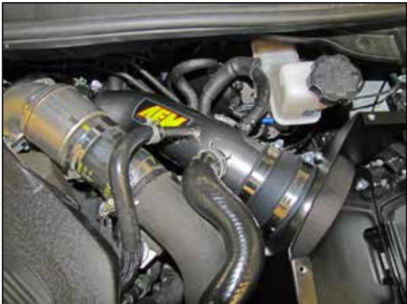
15. Connect the three vent hoses to the AEM® intake tube and secure with the factory spring clamps.
