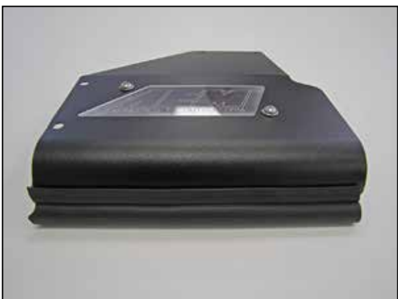
18. Install the edge trim into the heat shield lid as shown.
